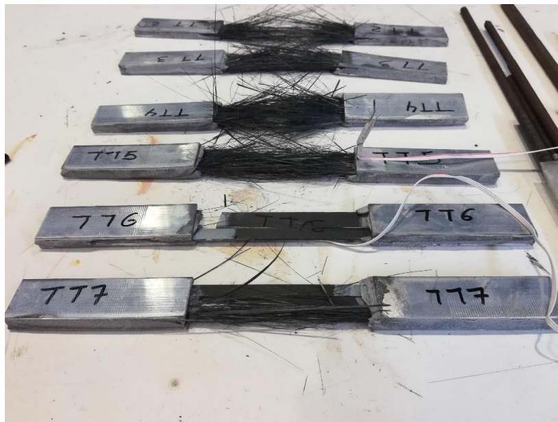
Figure 4: CFRP specimens at failure
