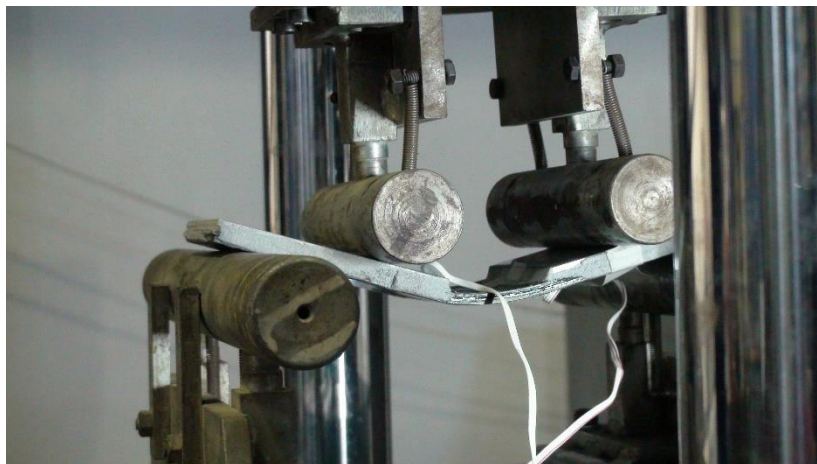
Figure 22: Test set-up for the 4-point bending test – CFRP in compression
