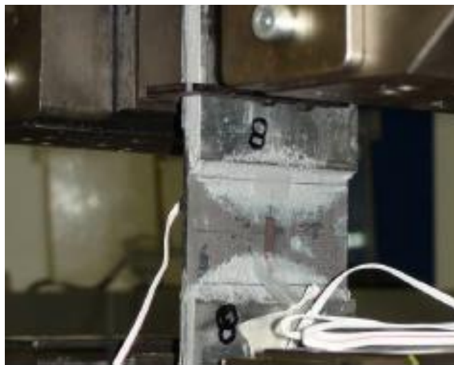
Figure 7: Test set-up for the tension test
